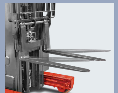
Forks can tilt forward/backward for easy loading
