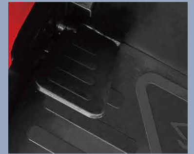
Safe pedal: when the pedal is released, traveling is stopped, and only hydraulic operation is enabled
