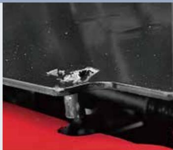
Integral locking pin structure on the baseboard can be opened without tool, which is convenient for daily repair and maintenance.
